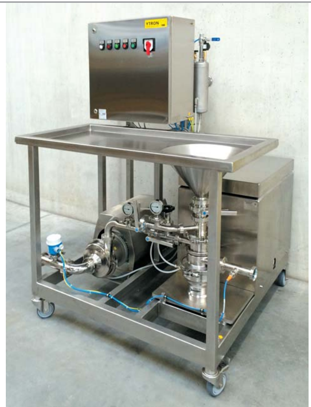
YTRON-ZC powder dispersion table in ATEX design Application: Dispersion of various powders for the Beverage Industry
