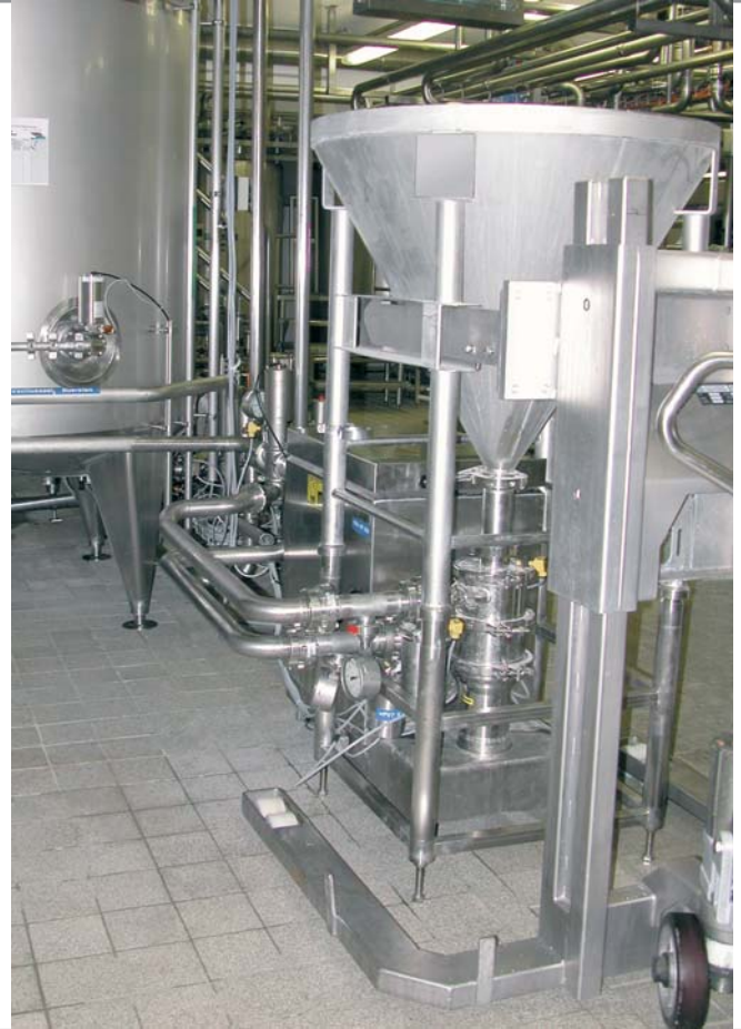
YTRON-ZC powder dispersion table in ATEX design Application: Dispersion of various powders for the Beverage Industry
